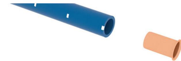
Insert the support sleeve into the pipe as far as it will go.
