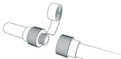
Metal threaded fittings must be used for permanent threaded connections. Threading plastic elements is prohibited. The threads are sealed with Teflon tape, sealing thread or special sealants.
