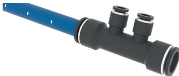
After assembly, it is possible to rotate the joint and after pressing the circlip, the pipe can be extended. When reassembling, the pipe must be relubricated and inspected for damage.
