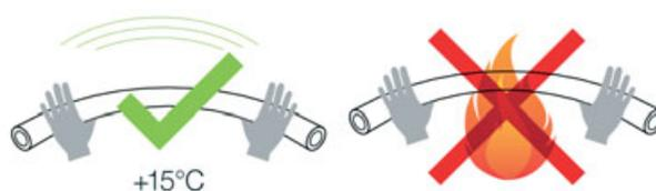
Pipe bending is performed without heating at a temperature of at least + 15 °C. For pipes with a diameter of 16 - 32 mm, the minimum bending radius is 8 times the pipe diameter (D).
