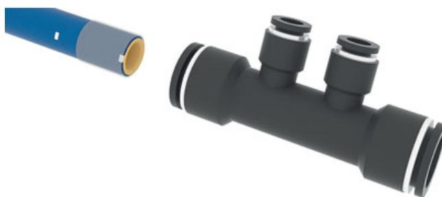
The fitting slides onto the pipe as far as it will go. Pipe 16 is inserted 27 mm, pipe 8 is inserted 20 mm. Marks printed on the pipe are used for orientation.
