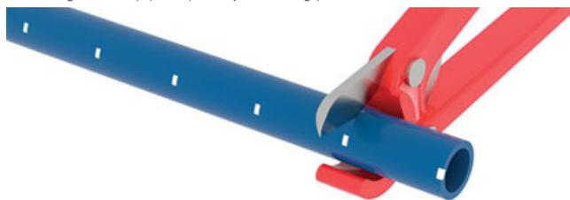
The pipe is cut with scissors perpendicular to the pipe axis. To prevent the pipe from flattening, it is advisable to turn the pipe using scissors.
